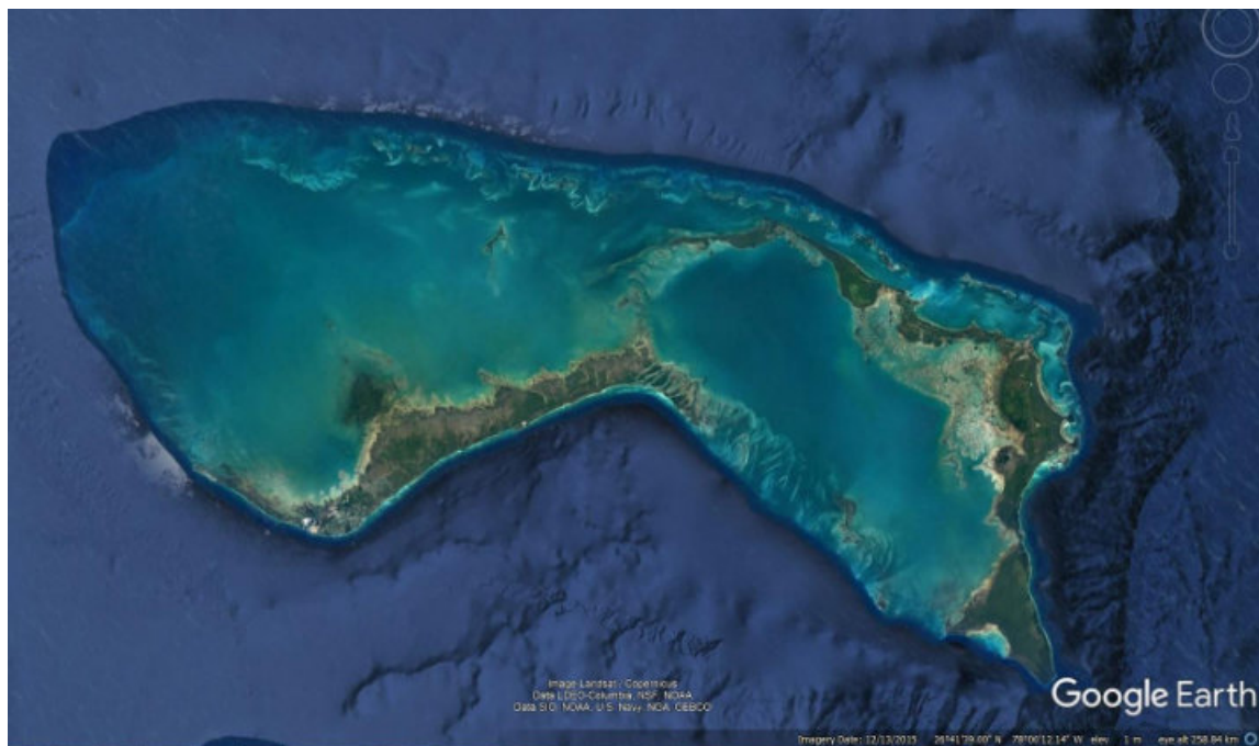
Fig 40 Present-day carbonate banks, Bahamas. Google Earth vertical view. This is a good analog for past carbonate platforms such as the Tuxpan Platform, Mexico, home of the famous Faja de Oro/Golden Lane hydrocarbon trend. Data © 2021 LDEO-Columbia, NSF, NOAA, SIO, U.S. Navy, NGA, GEBCO. Image © 2021 Landsat/Copernicus.
